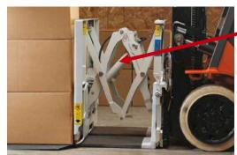
Using the Pull Tab pull the load back onto the forklift
