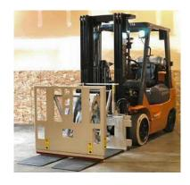
Push/Pull Attachment must be fitted to the Forklift
